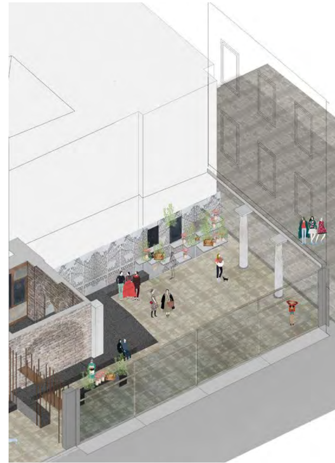
Isometric view of panellised wall system, with folding platforms for flower display and storage, and plinth market furniture for charity stalls.
