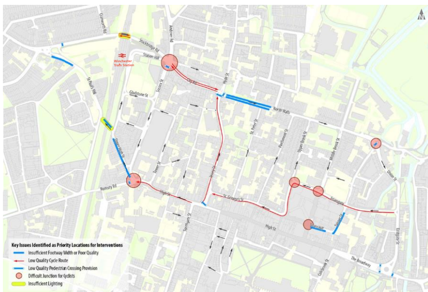
Fig. 10 - Priority areas for intervention based on PERS - Pedestrian Environment Review System and Cycling Level of Service Assessment (CLoS) assessments. Source: Atkins
