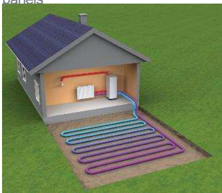
Ground Source Heat Pumps
