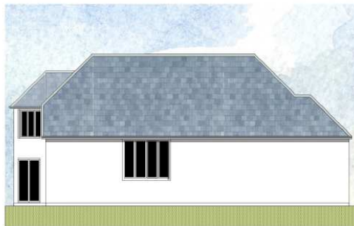
The roof is natural slate Windows and doors are painted softwood timber North West Elevation
