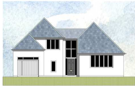
The roof is natural slate Windows and doors are painted softwood timber South West Elevation
