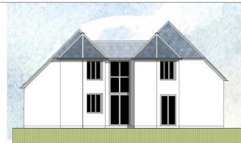
The roof is natural slate Windows and doors are painted softwood timber North East Elevation
