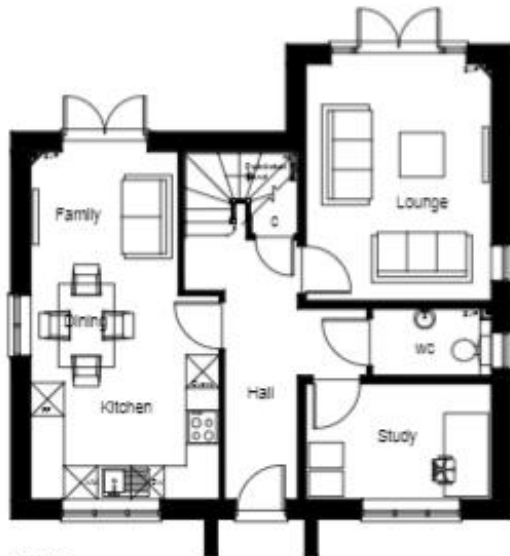
PLOT 3 GROUND FLOOR PLAN (1:50)
