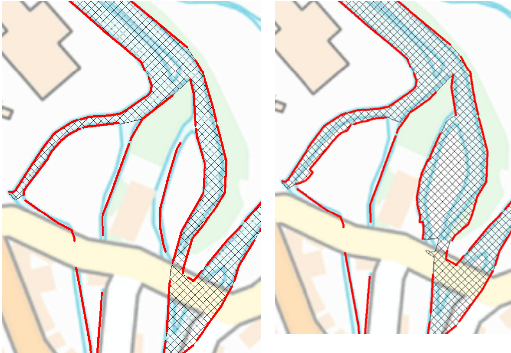
Figure 10: Original (left) and updated (right) 1d-2d connections (red) showing area excluded from 2d TUFLOW model as modelled in 1d (hatched). Note all channels shown are modelled in 1d model.
