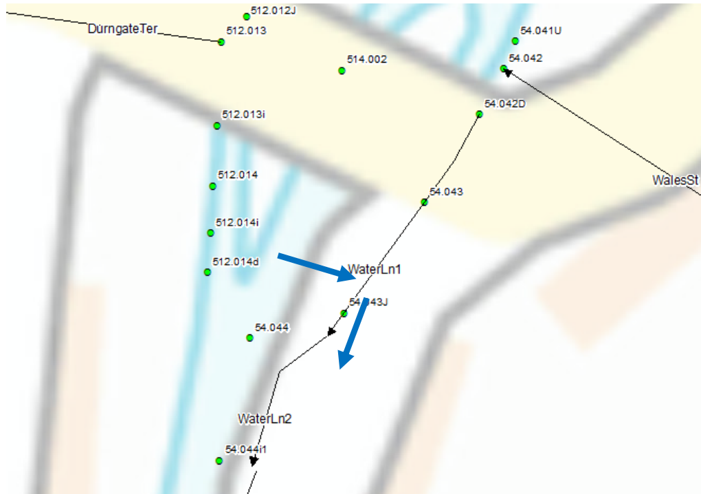
Figure 17: Location of initial overtopping (indicated by blue arrows) along Water Lane north of flood defence wall.
