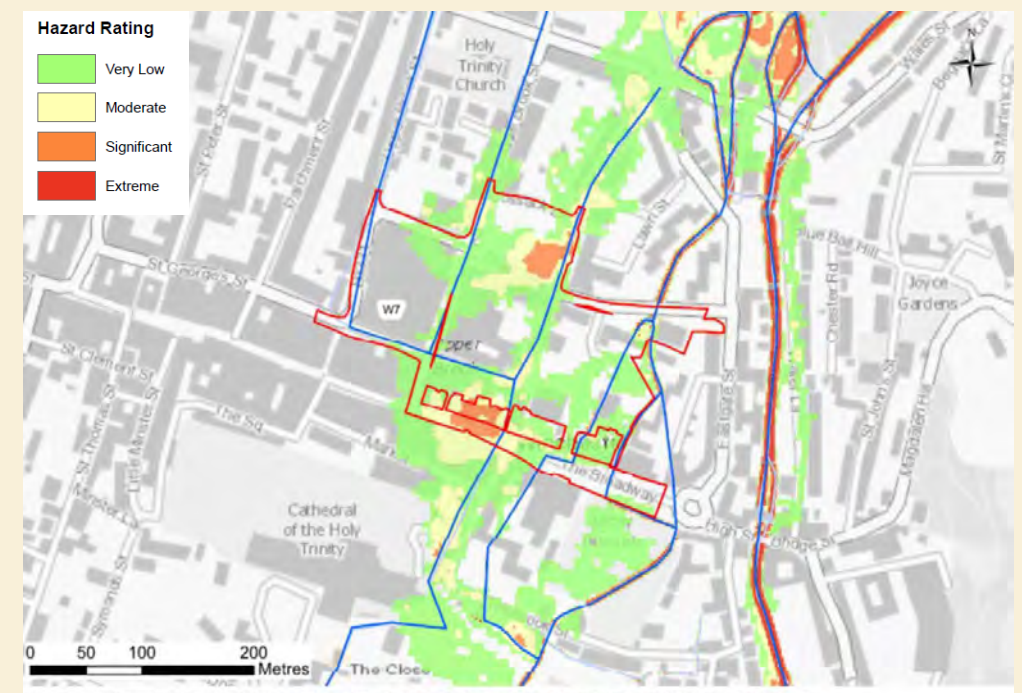
Figure 24: Hazard mapping for the 1:100 year + 35% modelled flood events [7]
