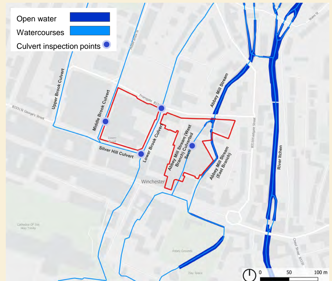
Figure 20: CWR site map, culverted and open watercourses
