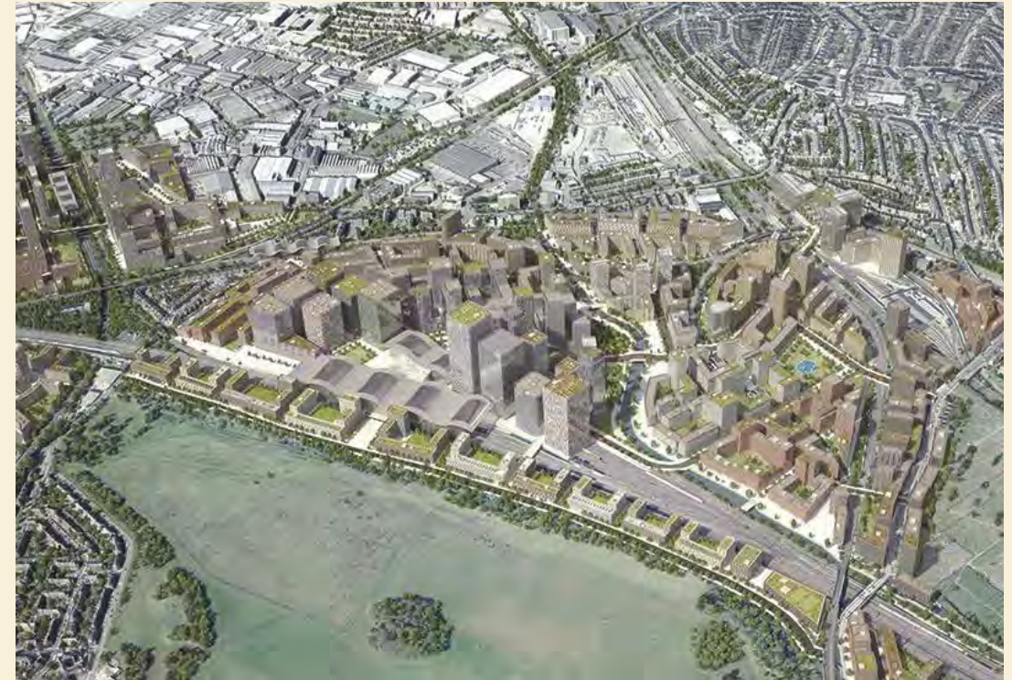
Figure 35: Old Oak West Masterplan, West London Old Oak West masterplan aims to deliver 10,000 new homes in West London in an area with very limited sewer capacity. The design approach taken maximises diversion of stormwater from the sewer system by maximising direct discharge to the Grand Union canal to free up capacity for foul water drainage flows.
