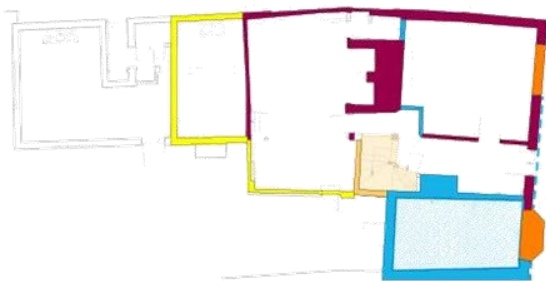
c.1840 Fenestration changes including the addition of the angular bay to the front elevation
