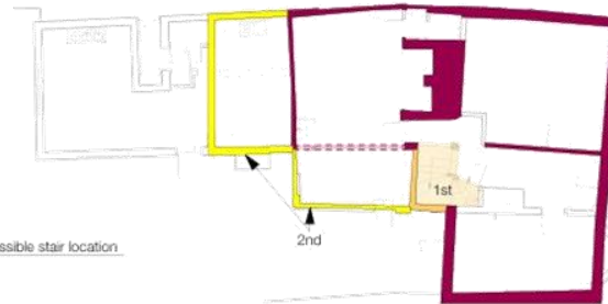
c.1670-1690 Modifications made including addition of stair tower and extensions/areas of rebuilding after the Airstord fire of 1689
